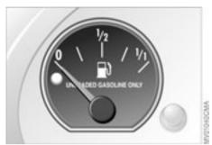
Once the indicator lamp stays on continuously, there are still approx. 2 gallons/8 liters of fuel in the fuel tank.
